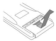
2 Insert two AAA batteries with the correct ± orientations.
